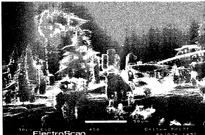
Fig. 1. An electron microscope picture of KCl crystal spires condensed from gas at 550C.
