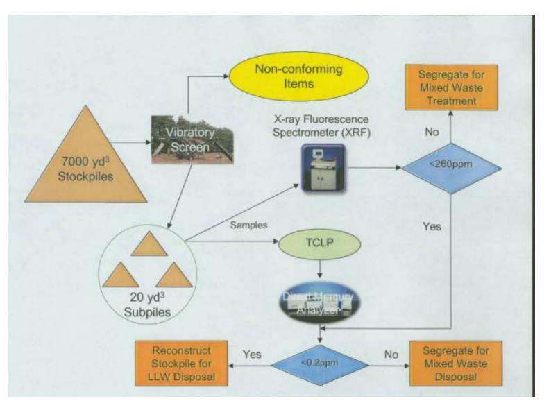
Figure 1. Sorting and analysis flow diagram for Field Laboratory
