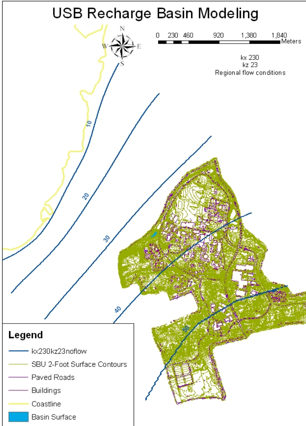
Figure 3. Initial model of regional flow conditions, assuming standard conductivities for the Upper Glacial aquifer: horizontal conductivity of 230 feet per day, vertical conductivity of 23 feet per day, and with no input from the recharge basins.
