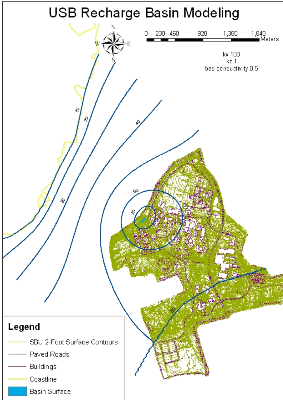
Figure 6: 10' interval water table contours, assuming local conductivities for Upper Glacial aquifer: horizontal conductivity of 100 feet per day, vertical conductivity of 1 foot per day, unlimited flow into the basins, and with conductivity of basin floor sediments of 0.5 feet per day.
