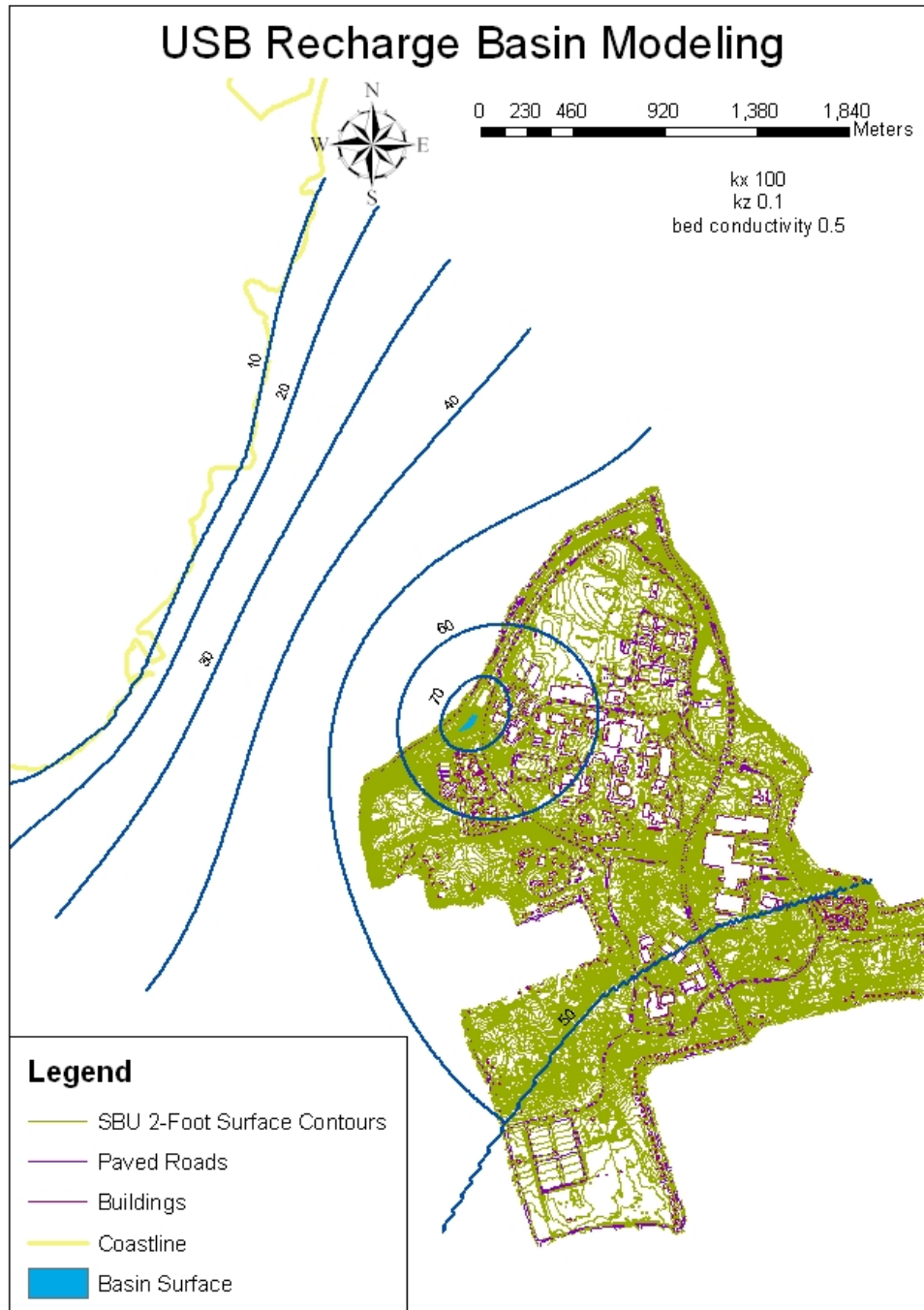
Figure 7: 10' interval water table contours, assuming local conductivities for Upper Glacial aquifer: horizontal conductivity of 100 feet per day, vertical conductivity of 0.1 feet per day, unlimited flow into the basins, and with conductivity of basin floor sediments of 0.5 feet per day.
