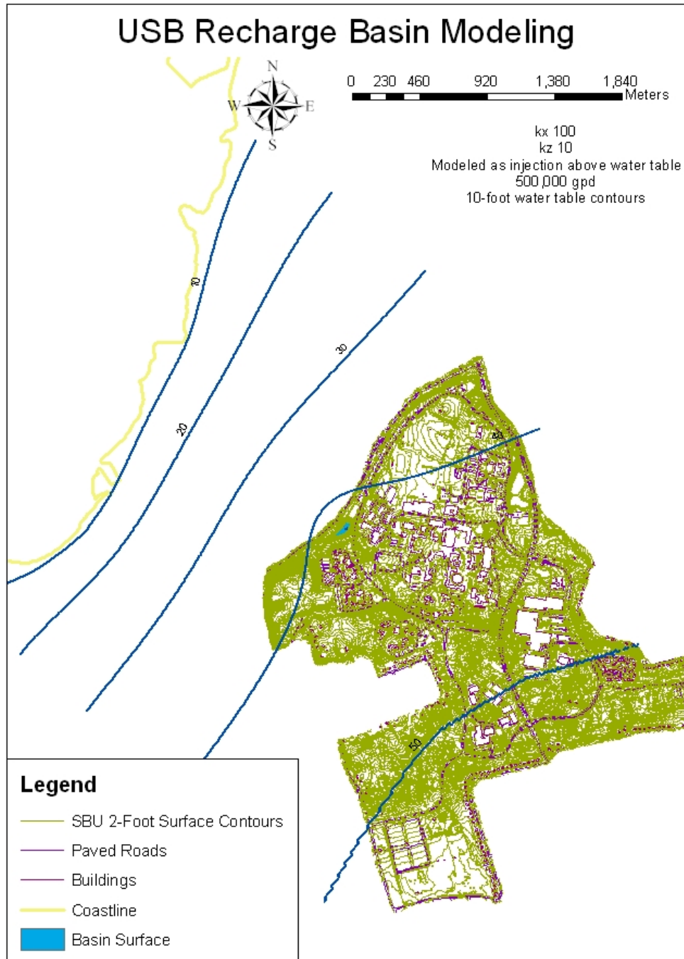
Figure 13: 10' interval water table contours, assuming acceptable conductivities for Upper Glacial aquifer: horizontal conductivity of 100 feet per day, vertical conductivity of 10 feet per day, and a flow out of the basins of 250,000 gallons per day. The center of the mound is approx. 17' higher than the regional water table.
