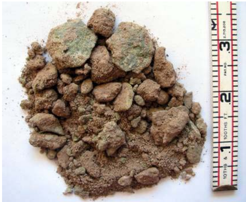
Figure 6. Sample from Boring B of main study site at the base of the upper varved layer (asterisk in Figure 5 at elevation -15') of disturbed and dried out till containing gravel sized pieces of serpentinite. Ruler is graduated in tenths of feet.
