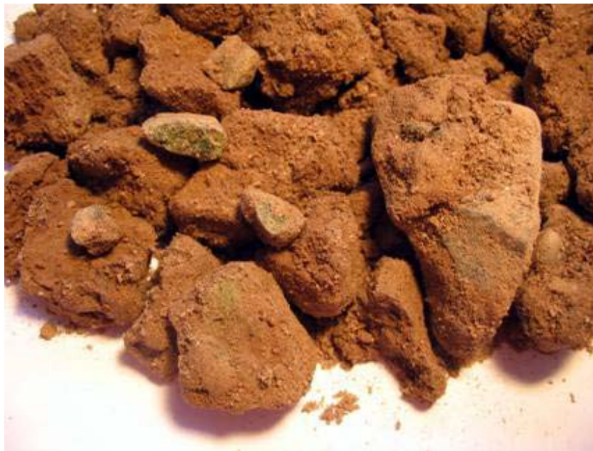
Figure 8. Sample of till from Boring E (asterisk in Figures 4 and 5 at elevation -19') from the base of the upper varved layer. Most of the soil structure was disturbed during the reclassification process and storage. Note the presence of coarse gravel and a few serpentinite pebbles in a red-brown silty matrix. The soil mass shows the mix of fine to coarse-grained sand tightly packed together with red-brown silt. Width of view is roughly 3 inches.
