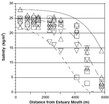
Figure 2. Salinity intrusion curves fitted to field data showing mixing of brackish water from the East River with freshwater from the upland end of the Flushing Bay watershed. Symbols indicate estimated tidal stages at sample collection locations (Eaton 2007)
