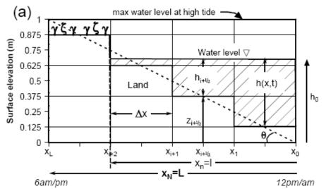
Figure 3. Conceptual model of a terraced constructed wetland profile from which hydraulic loading based on tidal fluctuation was used to estimate potential reduction of contaminants in coastal waters (Eaton and Yi, in review)
