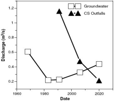
Figure 1. Changing trends of estimated freshwater discharges to Flushing Creek and Bay, data from USGS and NYCDEP (Eaton 2007)
