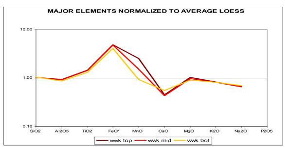
Fig. 4. Wildwood State Park loess normalized to average loess from Schentger , 1992. shows large enrichment in Fe and depletion in Ca. Ca is probably leached from the soil because Long Island soil is acidic.
