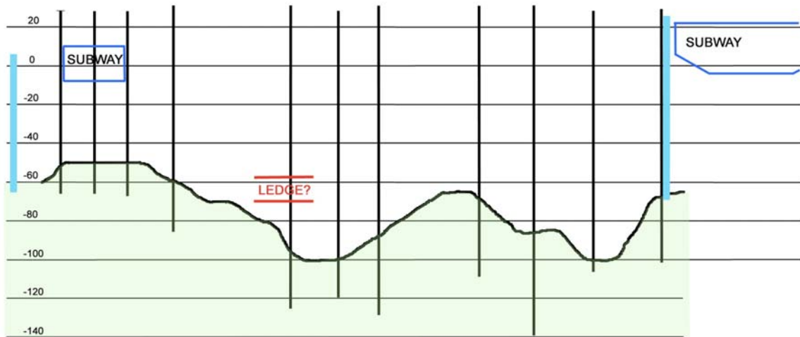
Figure 6 – Cross-section through the depressions in the east bathtub, facing north. Red lines show the location of either a ledge of bedrock or an 11 foot thick pegmatite boulder. Location of cross-section is shown in Figure 7. Elevation 0' is equal to El +2.653' on USGS Mean Sea Level Datum at Sandy Hook, NJ (1929 NGVD).
