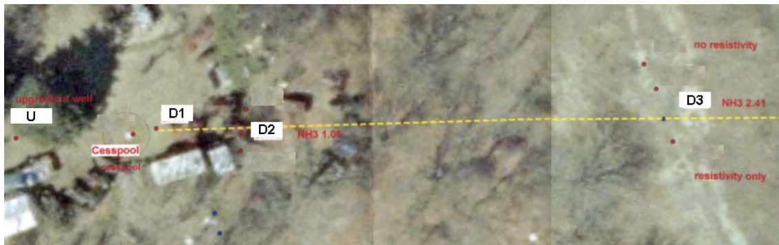
Fig. 4 Location of the site and positions of installed wells.
