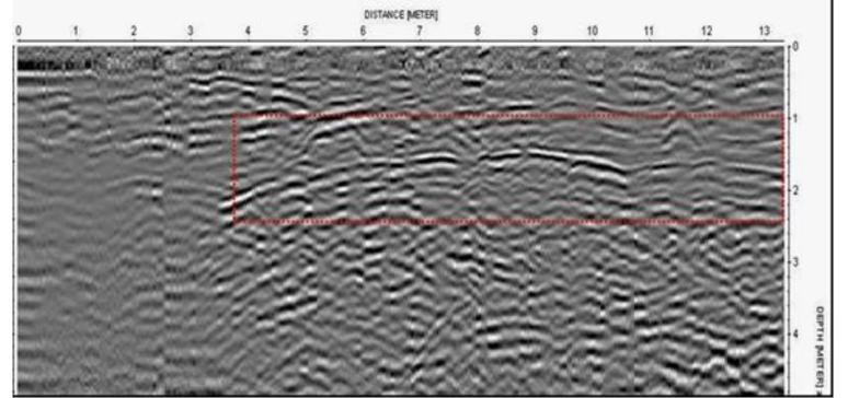
Fig. 3: 500 MHz radargram of the foundation at the Dune Road well field with vertical exaggeration removed. The foundation measures about 7 m (23') long and is about 2 m (6.5') deep in this radargram. The vertical scale is radar wave travel time (which has been converted to depth), and the horizontal is west-east (left-right) distance.
