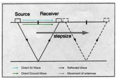
Fig. 2: GPR Basics: A short electro-magnetic wavelet is emitted by the transmitter. Portions of this wavelet travel directly through the air and along the surface (air and ground waves). The subsurface portion may be reflected and recorded by the receiving antenna, and the resulting signal is displayed graphically on a computer. After Hubbard et al., 2002.
