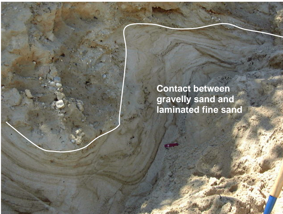
Figure 9. Fold found during construction of the Student Activity Center (SAC). The gravelly sands and finer, laminated sands and clay are folded. Swiss Army Knife is used for scale.
