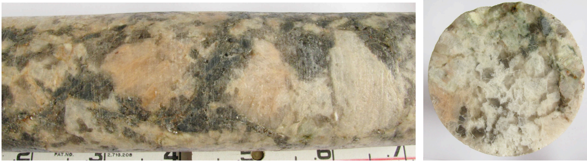
Figure 9 – Pegmatite. As an igneous rock, the crystals are interlocking and unfoliated. (Digital image by C. J. Moss.)
