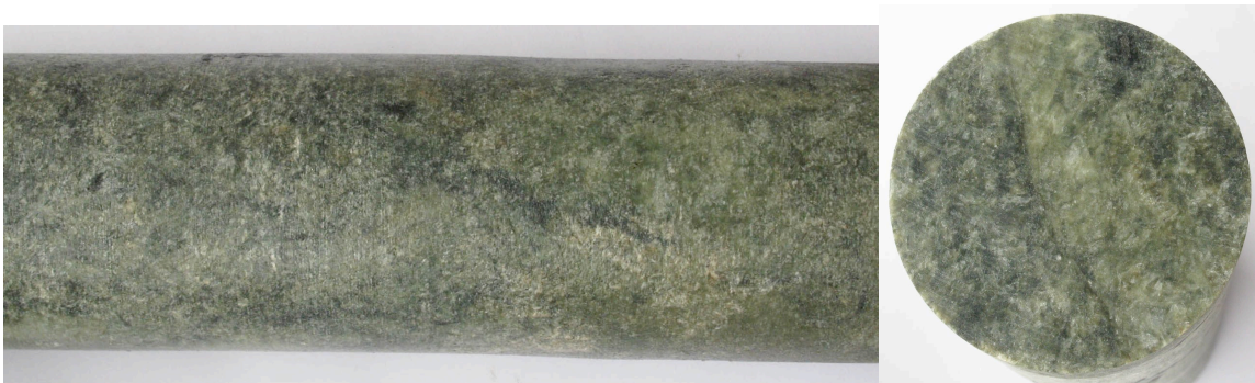
Figure 10 – Serpentinite. Serpentinite from near West and West 19 th Streets that was interlayered with Hartland schist. A neighboring site reported concerns with soft, highly micaceous and well-foliated rock (Altuntas and others 2008). (Digital image by C. J. Moss.)
