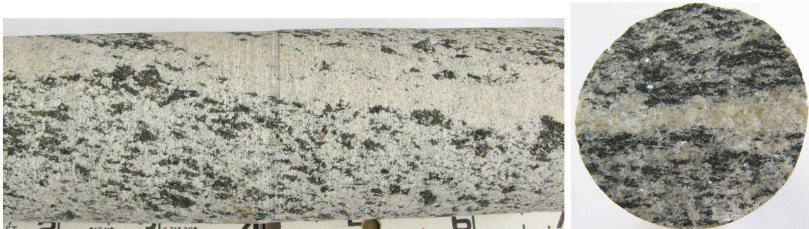
Figure 6 – Fordham Gneiss. – quite variable, but more often a gneiss than schist. (Digital image by C. J. Moss.)
