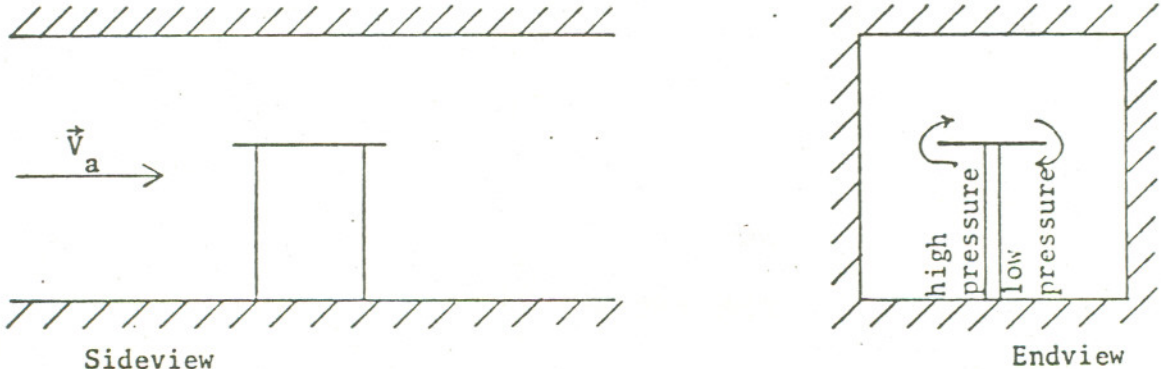
(c) "Leakage" Around Tip with Endplate (three-dimensional flow)
