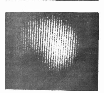
FIG. 8 SEPARATION OF MOIRE FRINGE FAMILIES WITH MASTER GRATING AT SECOND IMAGE PLANE
