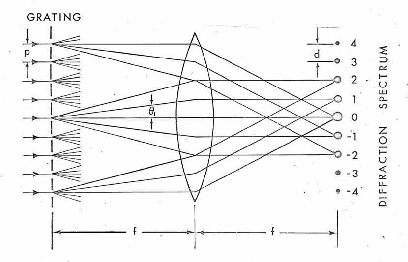
FIG. 3 IMAGE FORMATION MECHANISM OF THE DIFFRACTION SPECTRUM OF A GRATING
