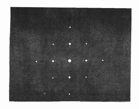
FIG. 5 PHOTOGRAPH OF THE DIFFRACTION SPECTRUM OF A CROSS GRATING (1000 LINES PER INCH)
