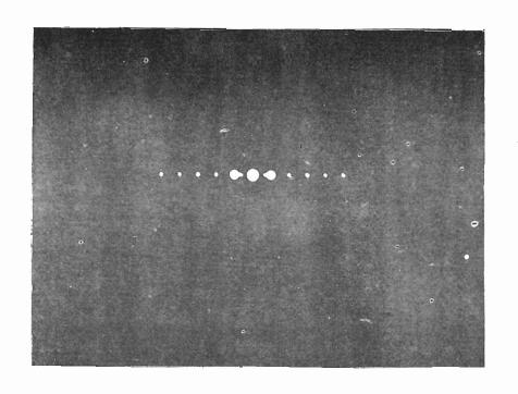
FIG. 4 PHOTOGRAPH OF THE DIFFRACTION SPECTRUM OF A LINEAR GRATING (300 LINES PER INCH)
