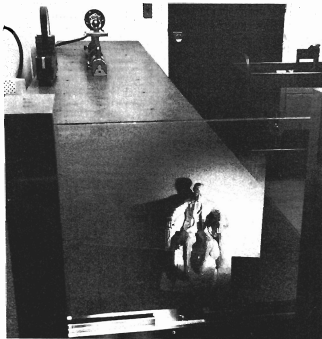
Figure 3 Three-dimensional virtual image as seen by looking through a bleached (transparent) phase hologram when it is illuminated by the laser in the back of it.
