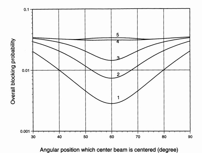
Figure 6. Overall blocking probability for different distributions of new call arrival rate concentrating at angular position of 60 degrees. It is plotted for C=15 and new call arrival rate/sector=0.1 calls/sed.
