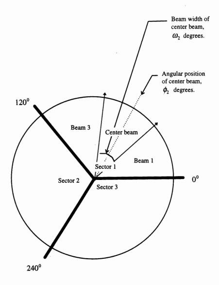
Figure 1. The system layout of sectorized multibeam cellular communication systems.
