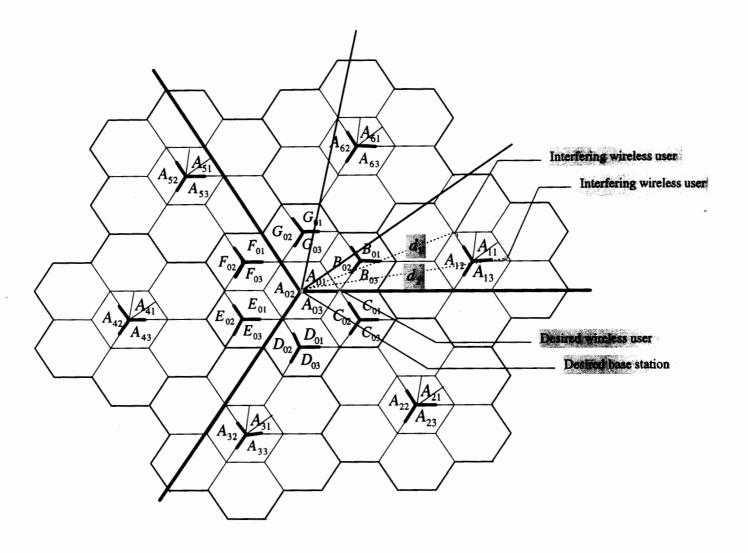
Fig 2 (a). 120°-sectored multibeam system with 3 beams in each sector for the up-link case. The cluster size is 7.
