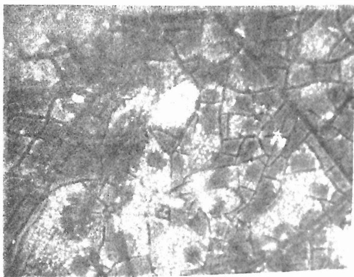
Fig. 4 E glass native surface after 48 hr. boiling in pH 2 oxalic acid solution. 240X
