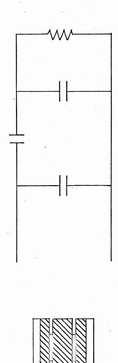
EQUIVALENT CIRCUIT OF CAPACITIVELY COUPLED DIPOLES IN TRANSMISSION LINE
