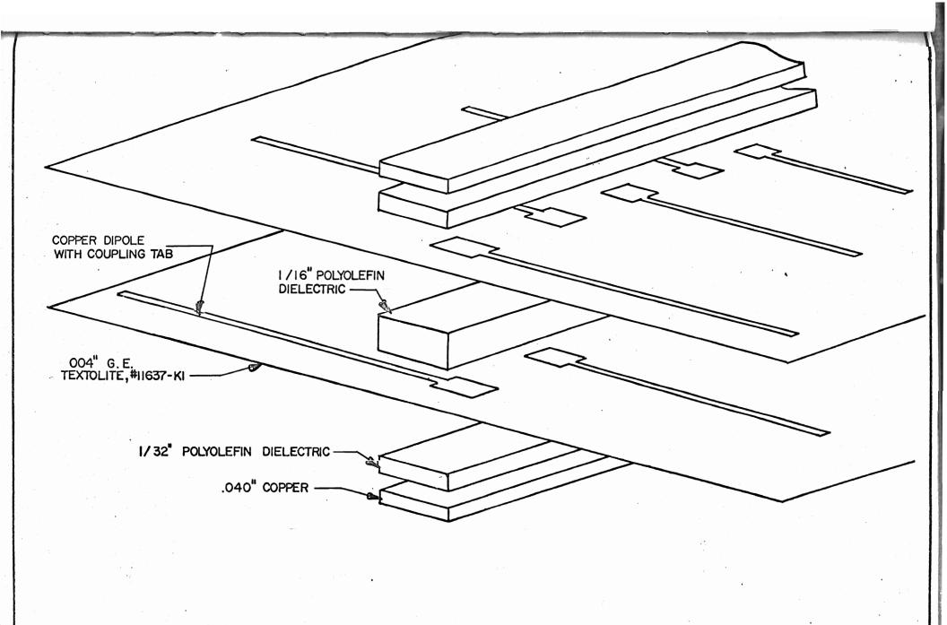
FIG. 2 EXPLODED VIEW OF PHOTO-ETCHED LOG-PERIODIC DIPOLE ARRAY
