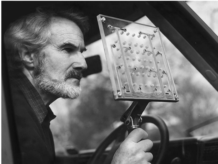
Fig. 7. The ISVR volume acceleration sensor (VAS) (photo).
