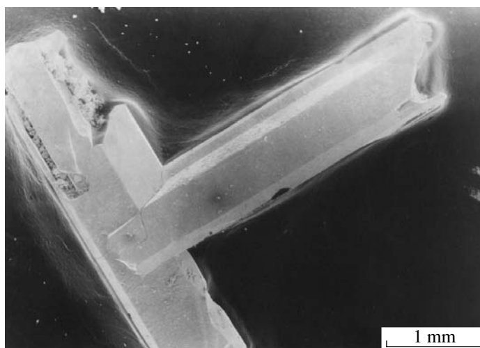
Fig. 2. Single crystals of \alpha -PbF 2 synthesized in the PbF 2 -KF-H 2 O system.
