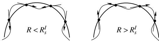
Fig. 4. Directions of tangential fluxes before and after the critical radius R_s^l .
