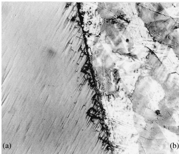
Fig. 1. The surface morphology of an epitaxial ZnO layer with a grain boundary grown on a (10\bar{1}2)\text{Al}_2\text{O}_3 substrate: (a) (11\bar{2}0)\text{ZnO} ; (b) (0001)\text{ZnO} (magnification, \times 350 ).
