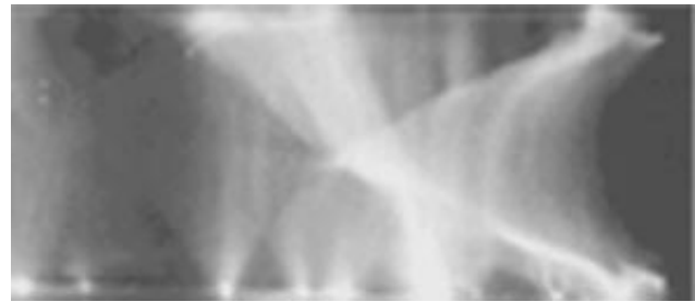
Fig. 4. Discharge glow in the unsteady flow behind the obstacles 70 \mu\text{s} after the passage of a plane shock with the Mach number M = 3.8 . The density of the steady gas flow behind the plane shock is 2 \times 10^{-5} \text{ g/cm}^3 .
