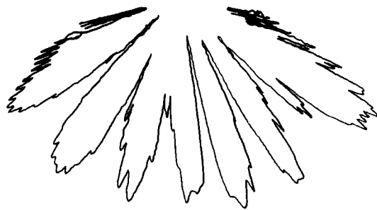
Fig. 12. Backscatter from a metallic Galois reflection phase grating shown in Fig. 11. (The measurements were made with 3-cm microwaves.)
