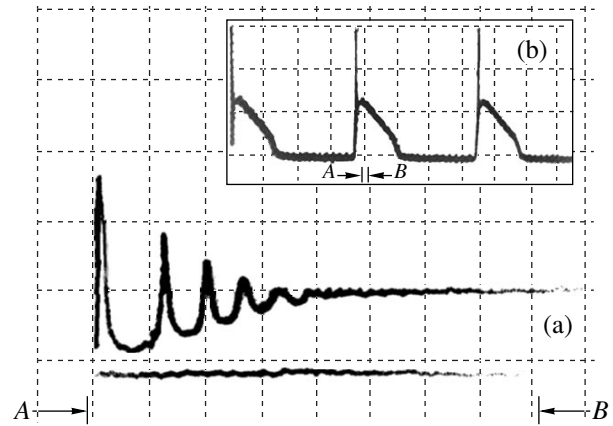
Fig. 9. High-frequency oscillations at the leading edge of the current pulse of a negative corona with a metal anode in nitrogen at P = 80 torr, R = 34 M \Omega , d = 30 mm, r_c = 0.1 mm, \langle I \rangle = 10 \mu A, and U = 1.0 kV: (a) a detailed structure of damping high-frequency oscillations that arise immediately after the leading edge of the current pulse (the time scale is 2 \mu s/division, and the current scale is 20 \mu A/division); (b) a general structure of low-frequency current oscillations (the interval A–B corresponds to high-frequency current oscillations shown in plot (a), the time scale is 100 \mu s/division, and the current scale is 20 \mu A/division).
