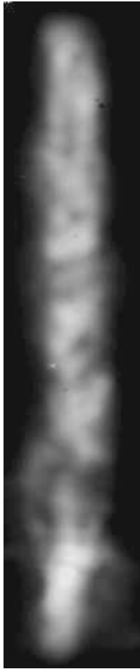
Fig. 8. Azimuthally axial inhomogeneities of the radiation of a pinch region; the pinch diameter is approximately 0.8 mm.
