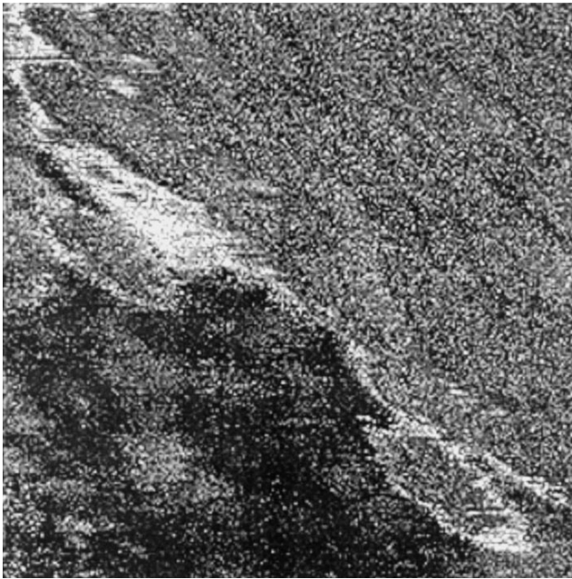
Fig. 2. A typical distribution of the surface sites with various values of the electron work function over a microscopic ( 90 \times 90 nm) area of a palladium–barium emitter surface measured with tunneling spectroscopy using a tunneling gap modulation technique. White, grey, and black regions correspond to an electron work function of 2.3 eV (minimum), \sim 3.7 eV, and 5.2 eV (maximum), respectively.
