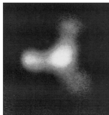
Fig. 1. Field-ion image of an adsorbed water molecule at room temperature.
