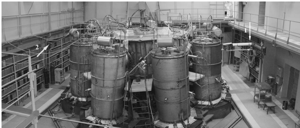
Fig. 1. General view of the S-300 facility. Arrow 1 indicates the photographic camera, and arrow 2 indicates the holder with mirrors directing the probing laser beams to the plasma object.
