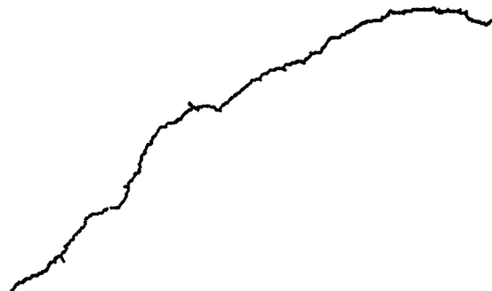
Fig. 4. A threadlike structure obtained using a modified DLA model with periodic “reset” of H ( L = 10 , H = 50 ).
