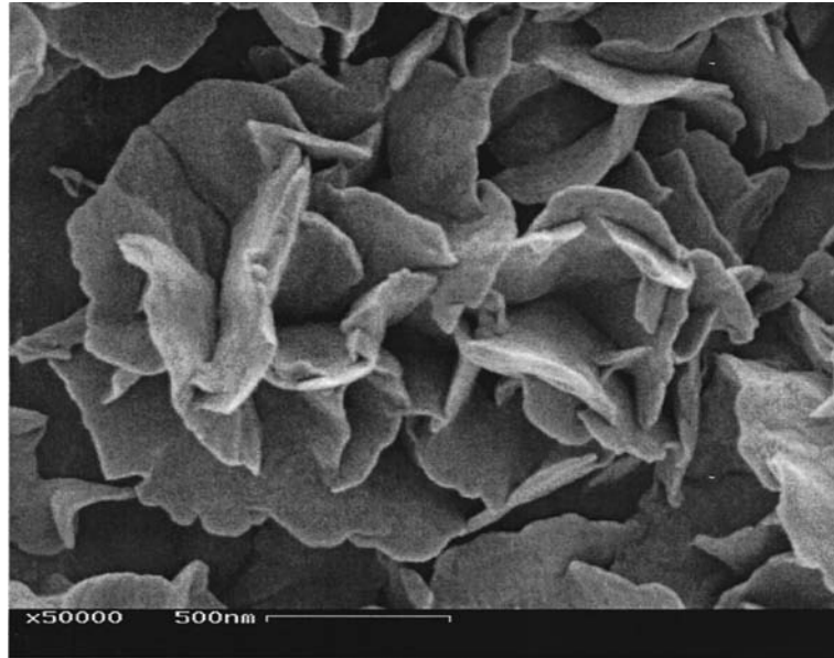
FIG. 2. Morphology of aged VC_{0.87} powder particles under \times 50\,000 magnification — the approximately 1\ \mu\text{m} particles consist of a collection of nanocrystallites in the shape of curved petals—disks ranging in diameter from 400 to 600 nm with a thickness of about 15–20 nm.
