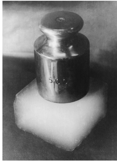
Fig. 3. SiO 2 aerogel with the mass density \rho = 0.15 g/cm 3 . The balance weight is 0.5 kg.
