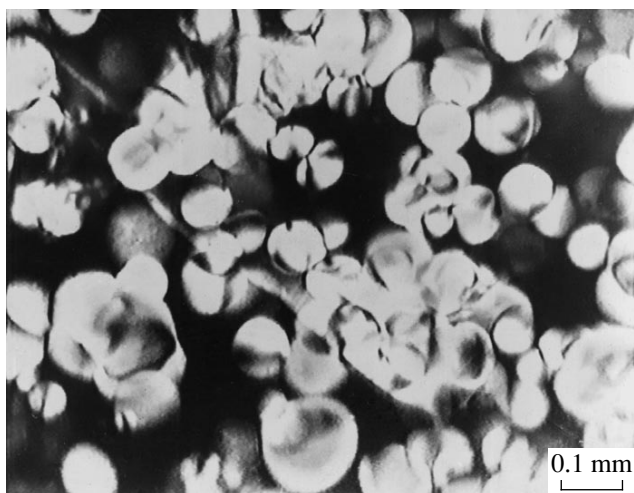
Fig. 4. Emulsion of flat liquid-crystal droplets in an isotropic medium which characterizes the G-1 state.
