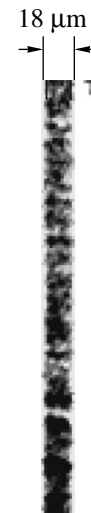
Fig. 7. Inner axial inhomogeneity of the core at the instant 60 ns after the beginning of the discharge. The current per wire is 30 kA. The liner with a diameter of 20 mm consists of 60 6- \mu\text{m} tungsten wires; the interwire distance is 1 mm.
