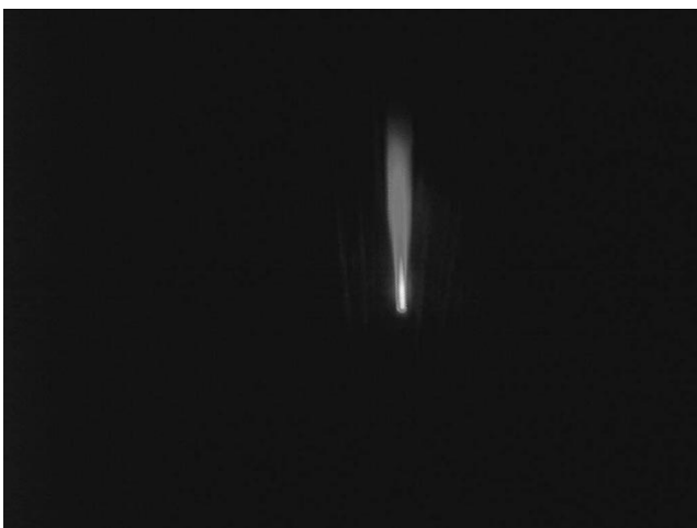
Fig. 3. Time-integrated photograph of a microwave torch. The working gas is argon.
