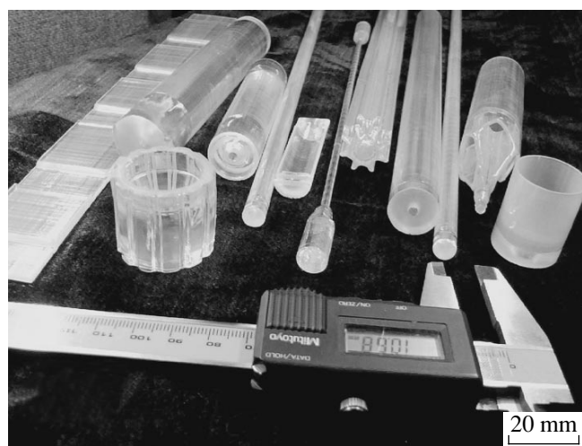
Fig. 3. Shaped crystals with varying cross section grown by the method of varied shaping.
