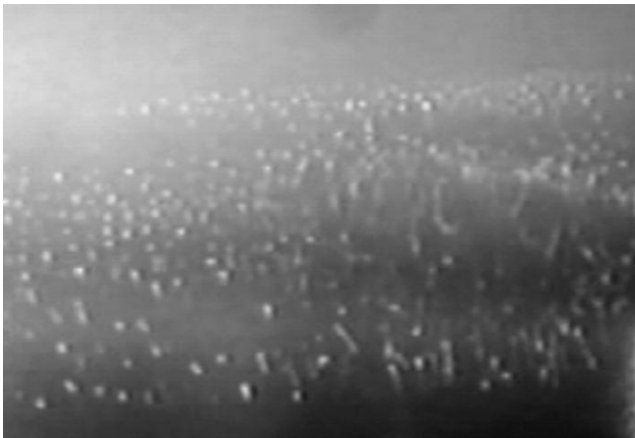
Fig. 18. Video recording of the dust self-oscillations in an rf discharge.
