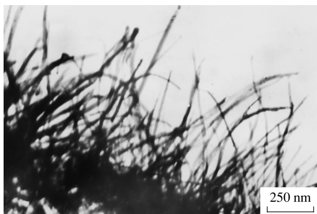
Fig. 5. \text{WO}_3 nanowhiskers at the early stage of their disintegration.
