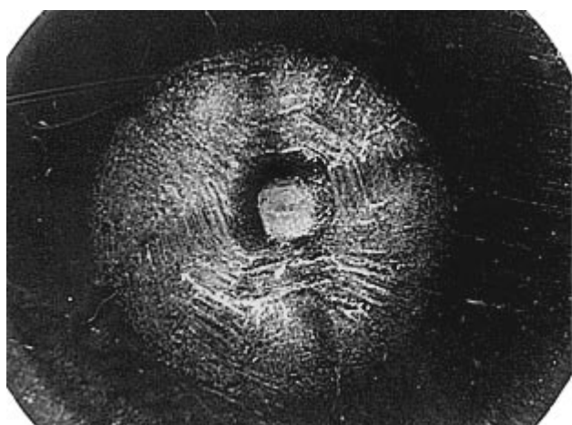
Fig. 3. Sectoriality in the distribution of bubbles. Dark areas correspond to the regions of the growth of the {110} faces of pyramids. The cut is perpendicular to the growth axis [110].
