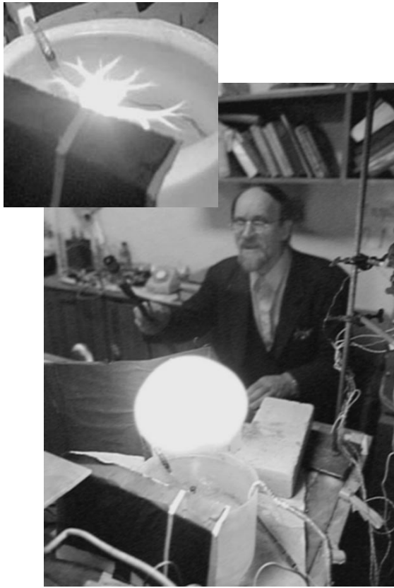
Fig. 1. Photograph of an LO. The inset at the top left of the figure shows a slipping discharge that preceded the appearance of a jet and its subsequent transformation into the LO.
