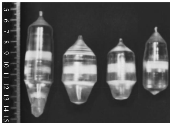
Fig. 4. Change in the character of the growth front (the ratio H/D ) with a change in the rotation speed of a crystal: (from left to right V_{rot} = 3, 15, 30, and 50 rpm). The temperature gradient above the melt is G = 70 K/cm.
