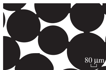
Fig. 1. Micrograph of PMMSs (polymer microspheres containing magnetic nanoparticles).
