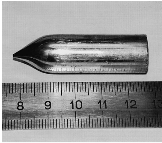
Fig. 3. Lead telluride crystal grown by the vertical Bridgman method with the introduction of axial low-frequency vibrations into the melt.
