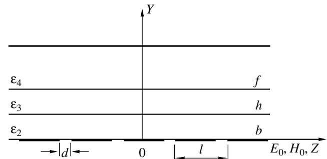
Fig. 1. Electrodynamic model of the distributed semiconductor structure.
