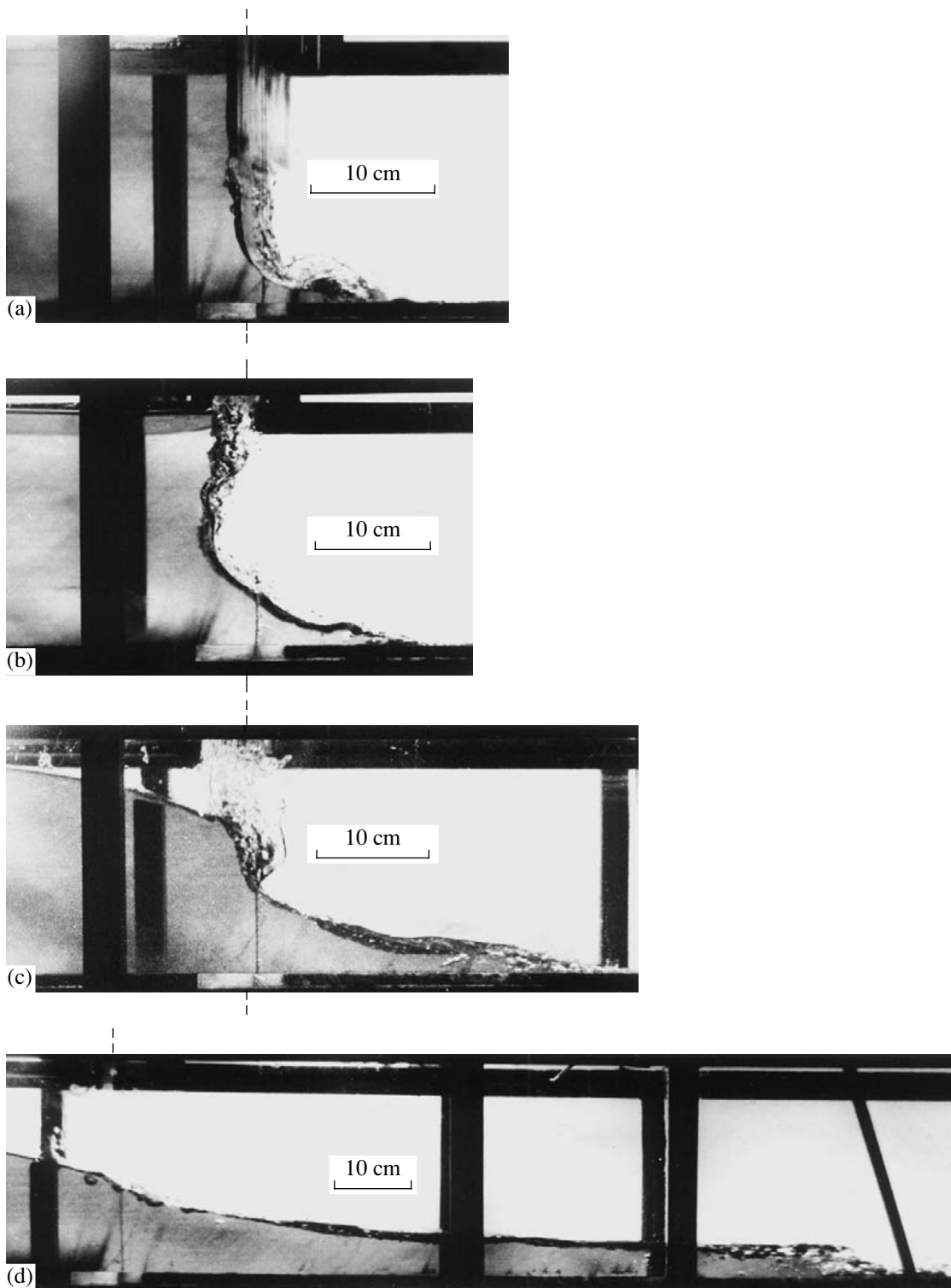
Fig. 1. Profiles of the free surface in the case of the dry bed in the tailwater, H_1 = 20.5 cm, H_2 = 0 , and t = (a) 0.03, (b) 0.05, (c) 0.18, and (d) 0.46 s. The vertical dashed line is the initial position of the gate.
