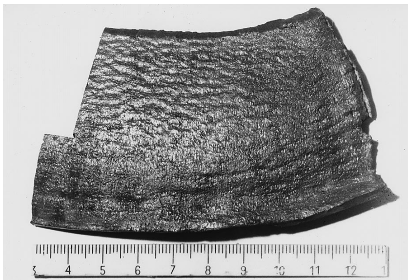
Fig. 2. Photograph of a fragment of the steel surface upon interaction with the explosion products.
