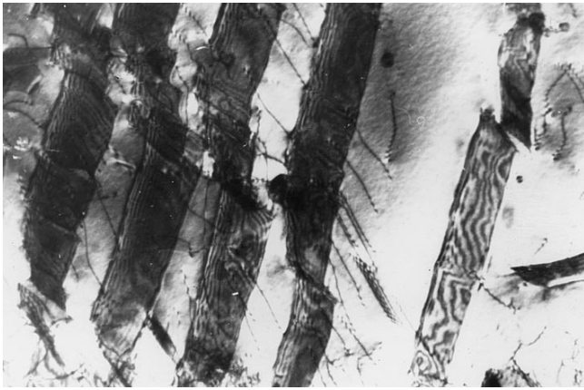
Fig. 2. Discontinuous decomposition after shock-wave loading, 1073 K, 1 h. A picture obtained with the use of an electron microscope, \times 40000 .
