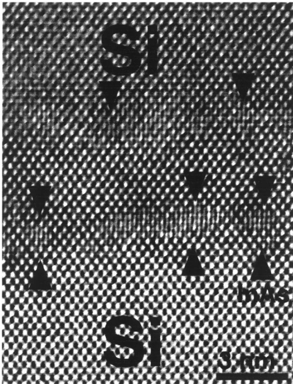
Fig. 5. Cross-sectional HRTEM image of sample B. InAs clusters are marked by arrows.
