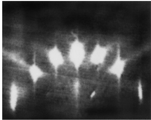
Fig. 1. RHEED pattern observed during epitaxial growth of monoisotopic silicon films. Direction of electron beam incidence: [011] ; energy of electrons in the beam: 10 keV.
