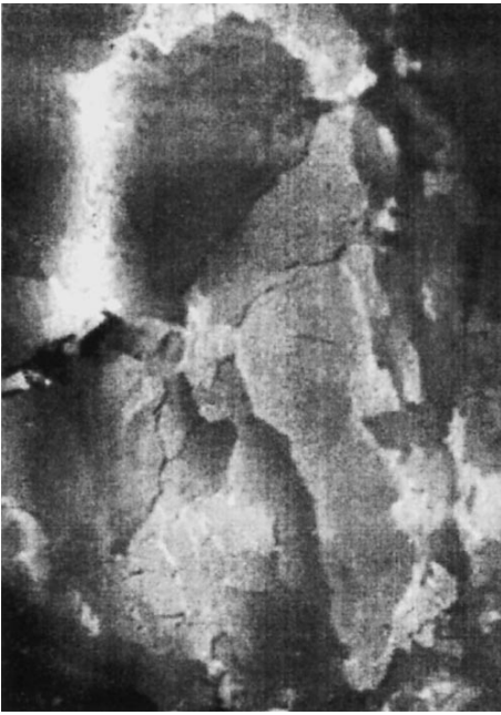
Fig. 1. X-ray topographic image of an MCMZT crystal in a (422) reflection. The magnification was \times 16 .
