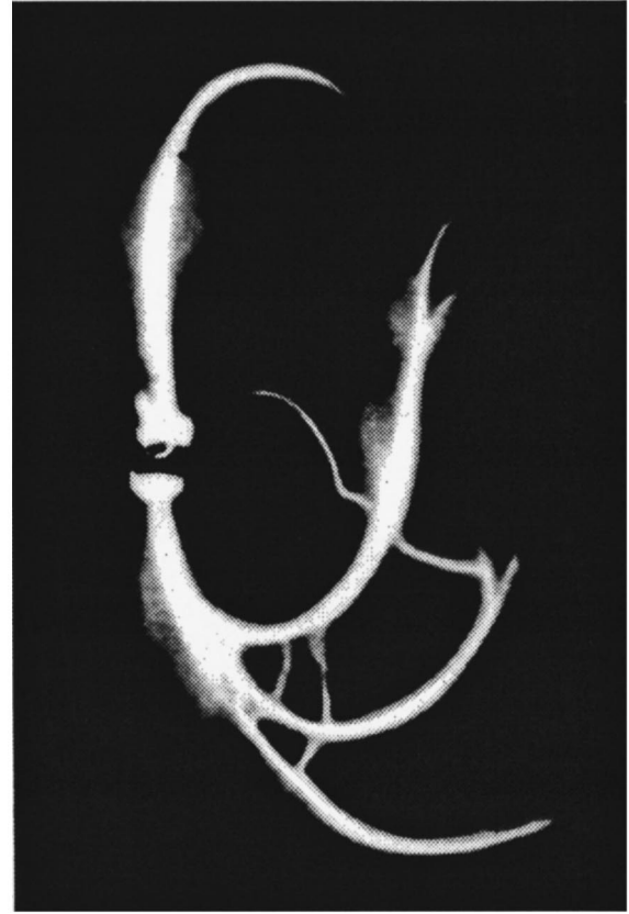
FIG. 5. Microwave discharge at p = 120 Torr, E_0 = 2.5 \text{ kV/cm} , and t_{pul} = 7 \mu\text{s} initiated by a sphere with 2a = 2.5 \text{ mm} .
