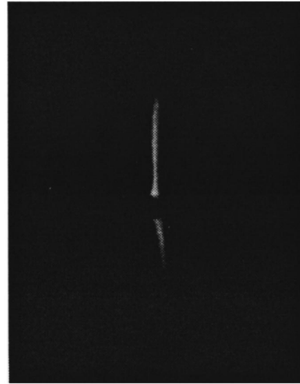
FIG. 4. Microwave discharge at p=30 Torr, E_0=1 kV/cm, and t_{\text{pul}}=7 \mu\text{s} initiated by a sphere with 2a=2.5 mm.
