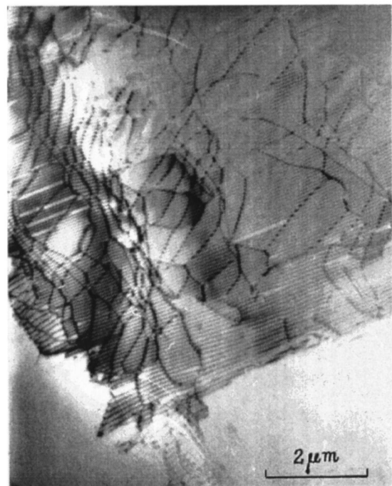
FIG. 6. Tilt subboundary in tungsten after rolling and annealing, RRR=200\,000 , 2300\text{ }^\circ\text{C} , \sim 3 s.
